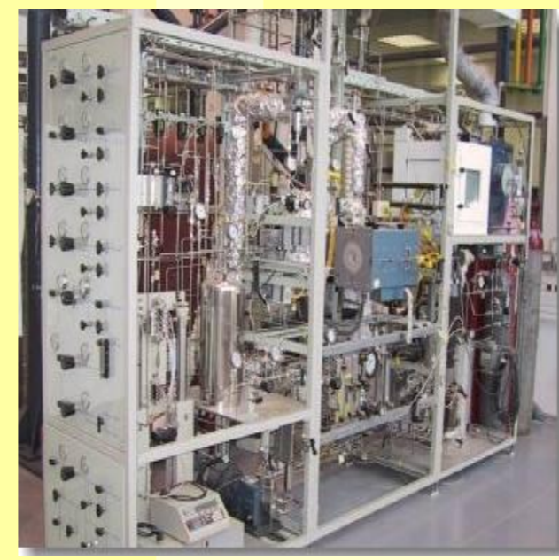
Catalytic steam reforming unit, CPERI, Greece
