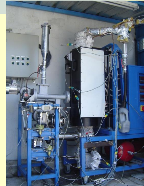
5 kW th pilot scale fluidized bed gasifier, AUTH, Greece
