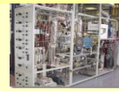
Catalytic steam reforming unit, CPERI, Greece
