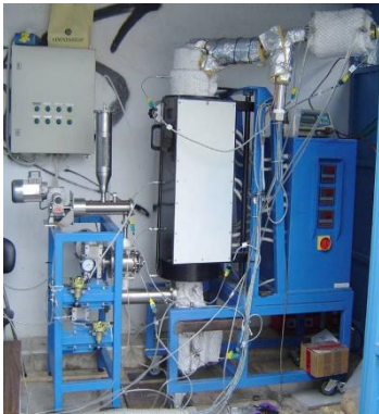
Pilot Fluidized Bed Gasification Unit (5kW th )
